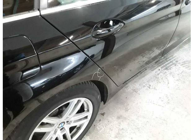
Damage #5: Side panel - rear right side: Side panel - Dent(s) - Smooth repair work
