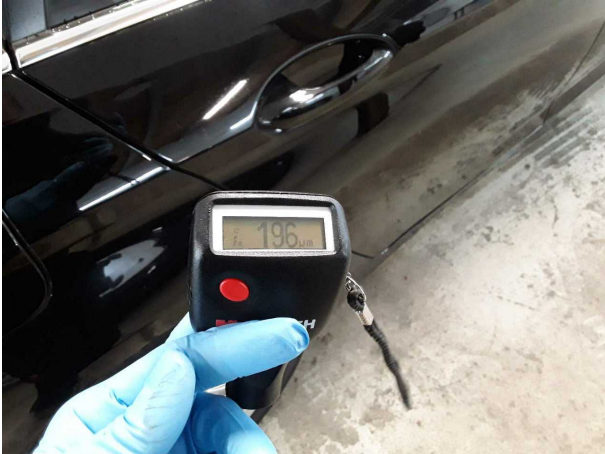
Repainting 1: Mudguard - right side, Sill - right side, Side panel - rear left side, Side panel - rear right side, Door - rear left side, Door
