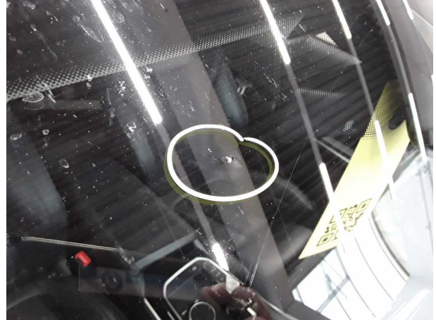
Damage #1: Vehicle glazing: Windscreen with lane departure assistant (mit Rissbildung zu nah am Rand) - Stone chips -
