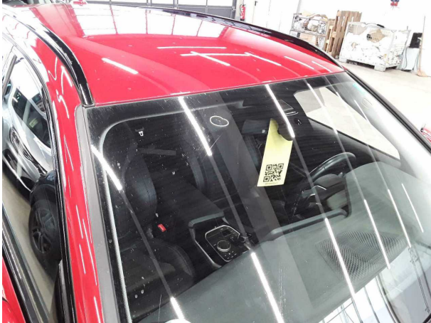
Damage #1: Vehicle glazing: Windscreen with lane departure assistant (mit Rissbildung zu nah am Rand) - Stone chips - Replace
