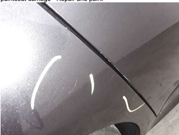
Damage #11: Side panel - rear right side: Side panel - Scratched - Repair and paint
