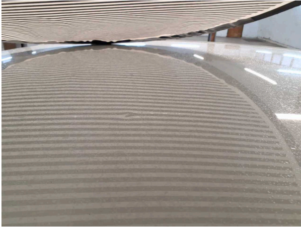
Damage 4: Roof: Roof - Dent(s) - Smooth repair work
