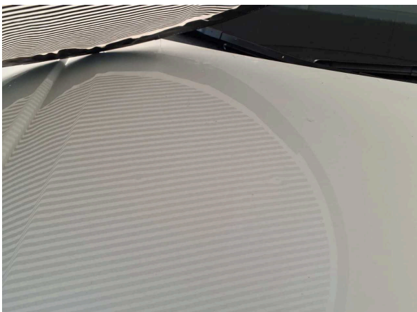
Damage 3: Bonnet: Bonnet - Dent(s) - Smooth repair work
