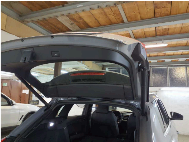
Damage #2: Boot lid / rear door: Gas pressure damper - Worn - Replace
