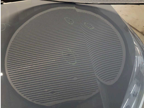
Damage #3: Bonnet: Bonnet - Damage by hail - Smooth repair work
