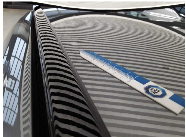
Damage #4: Roof: Roof - Dent(s) - Repair and paint
