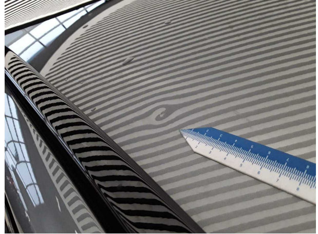
Damage #4: Roof: Roof - Dent(s) - Repair and paint
