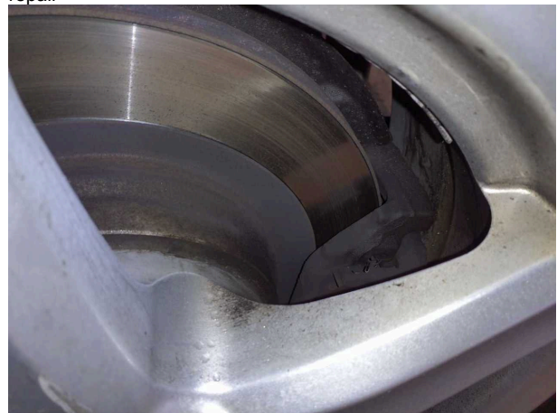
Damage #5: Braking system: Brake pads - rear - Worn - Replace
