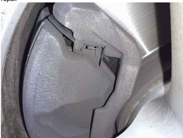
Damage #6: Braking system: Brake pads - front - Worn - Replace
