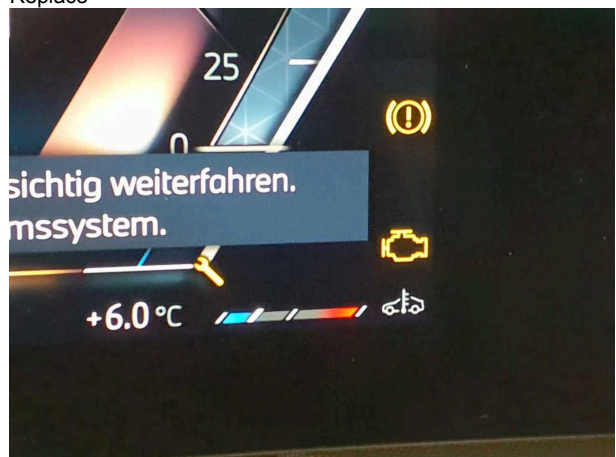
Damage #7: Electronic systems: Electronic systems (Motorkontrollleuchte an) - Due - Perform diagnosis
