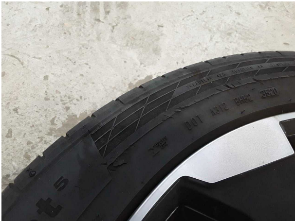
Damage #3: 2nd wheel set: 1 tyre - Damaged - Replace
