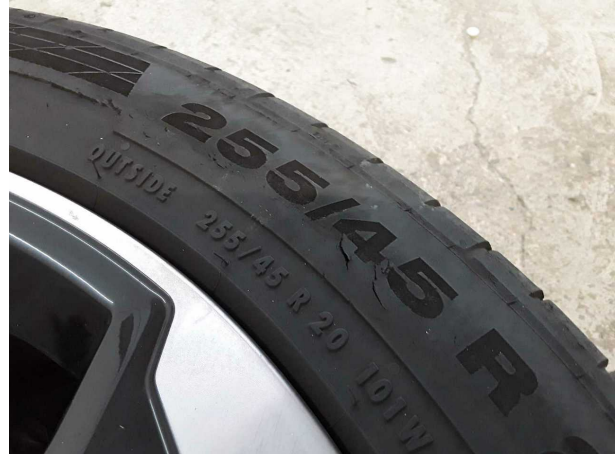
Damage #3: 2nd wheel set: 1 tyre - Damaged - Replace
