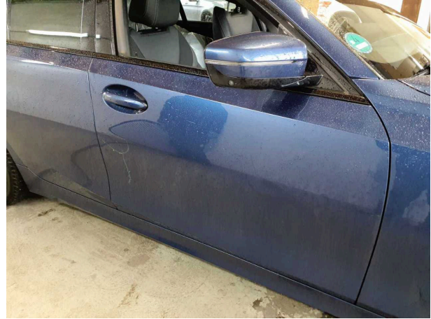
Damage #7: Door - front right side: Door - Scratched - Repair and paint
