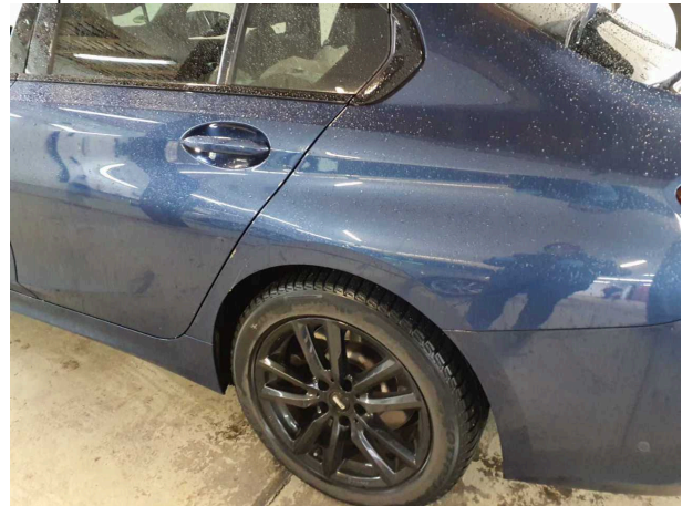
Damage #8: Side panel - rear left side: Side panel - Scratched - Repair and paint
