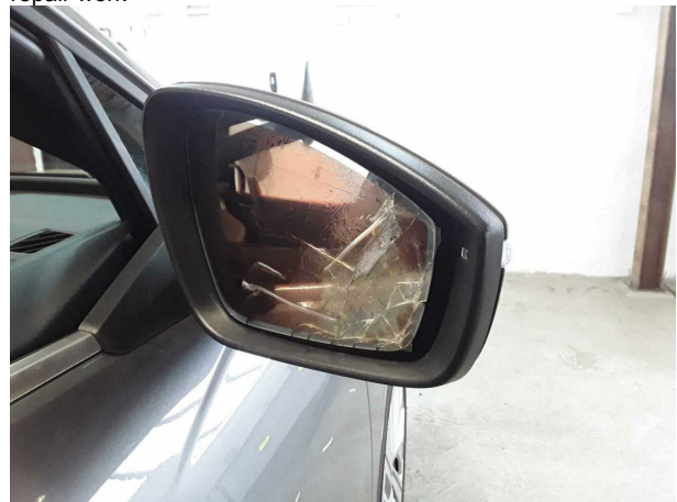
Damage #6: Wing mirror - right side: Mirror glass - Damaged - Replace
