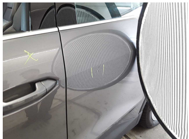
Damage #4: Door - rear left side: Door - dent(s) - Smooth rep... work
