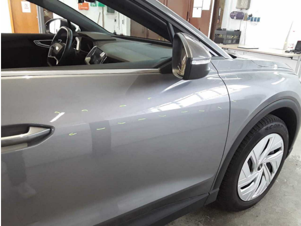
Damage #2: Door - front right side: Door - Scratch(es) - Cover / polish
