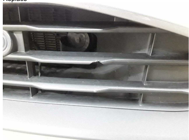
Damage #7: Front bumper: Air-inlet grille - Damaged - Replace
