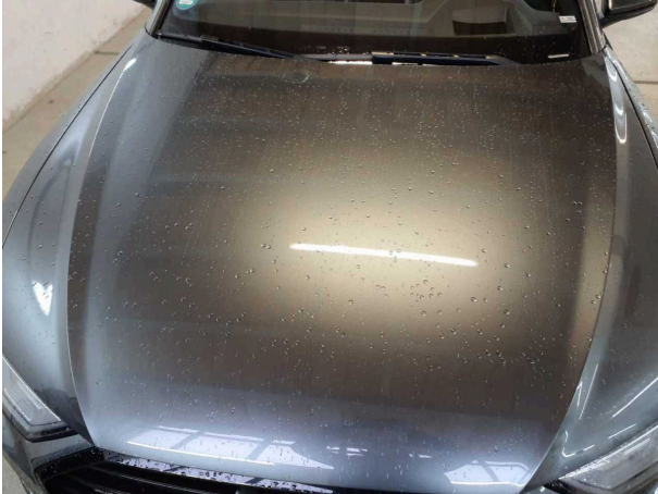
Damage #1: Bonnet: Bonnet - dent(s) - Smooth repair work
