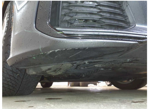
Damage #3: Front bumper: Front bumper - Scratched - Repair and paint
