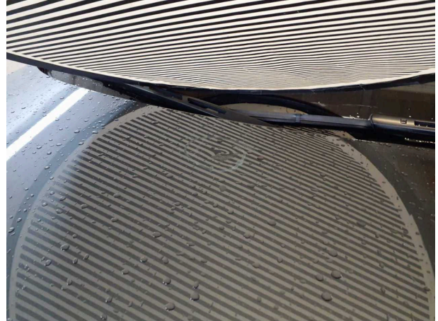
Damage #1: Bonnet: Bonnet - dent(s) - Smooth repair work
