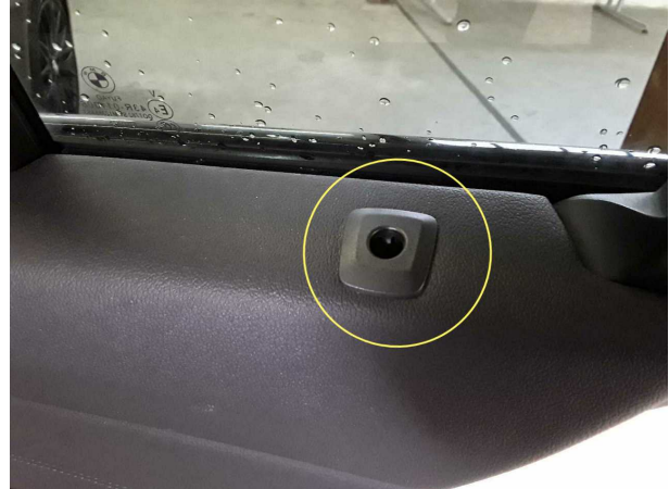
Damage #7: Trim / covers: Trim / covers (Stift Fehlt Tür hi re.) - Un- / install
