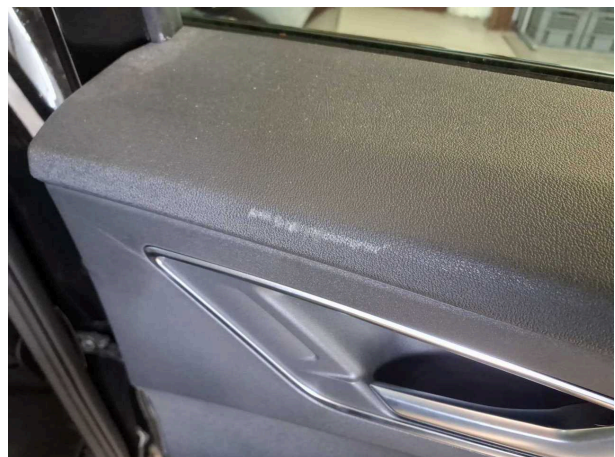
Damage 2: Trim / covers: Door trim - rear right side - Abrasio... Loss in value
