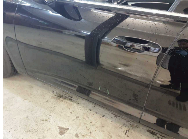
Damage #4: Door - front left side: Door - Dent / paintcoat damage - Repair and paint
