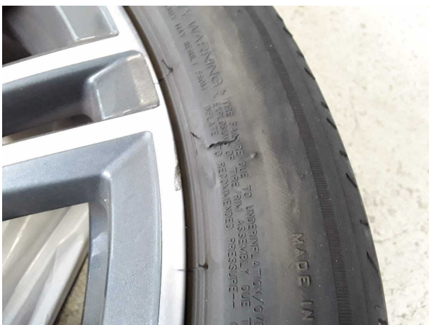
Damage #7: 2nd wheel set: 1 tyre - Damaged - Replace
