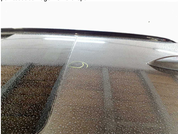
Damage #12: Roof: Roof - Dent(s) - Smooth repair work
