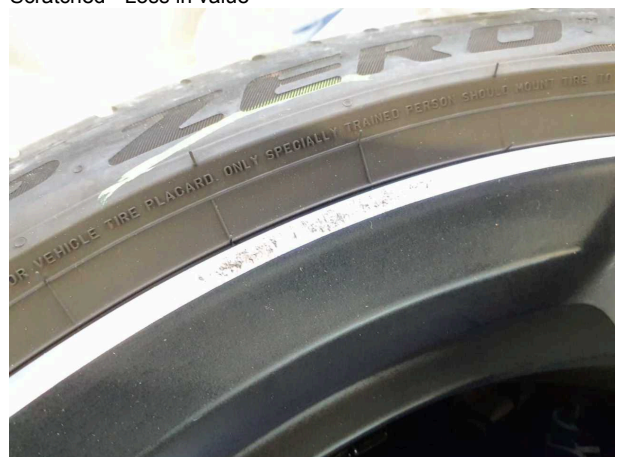
Damage #14: 2nd wheel set: Alloy rim set - complete - Scratched - Loss in value
