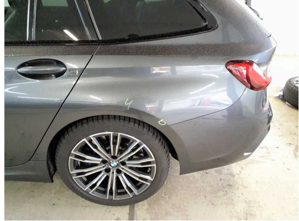
Damage #11: Side panel - rear left side: Side panel - Dent / paintcoat damage - Smart repair
