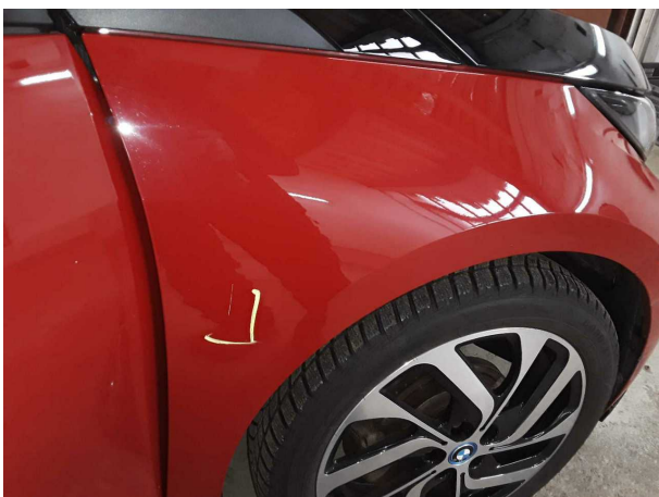
Damage #9: Mudguard - right side: Mudguard - right side - Scratched - Repair and paint
