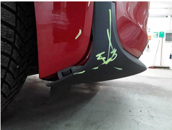
Damage #13: Front bumper: Front bumper - Damaged - Replace
