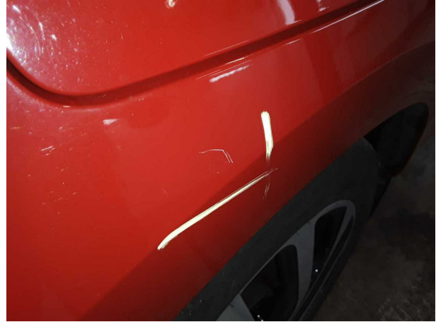
Damage #12: Side panel - rear right side: Side panel - Scratched - Repair and paint
