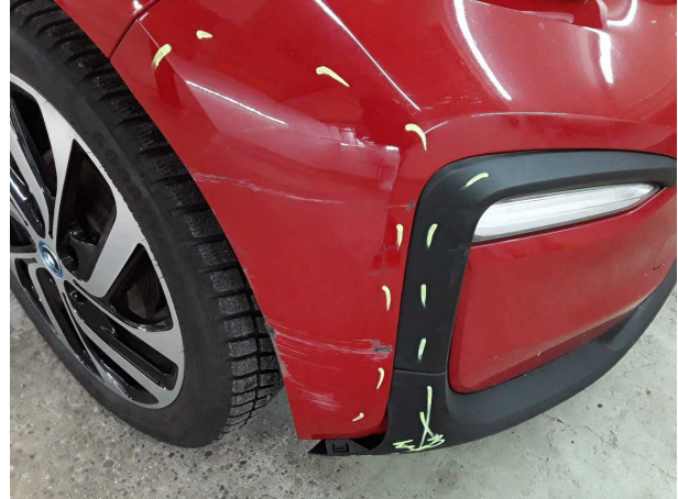
Damage #13: Front bumper: Front bumper - Damaged - Replace
