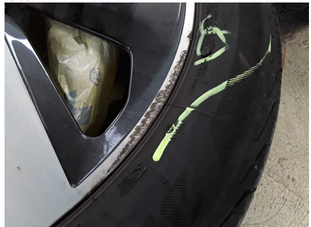
Damage #5: 2nd wheel set: 1 alloy rim - Scratched - Loss in value
