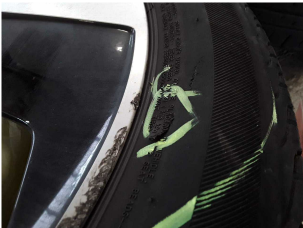
Damage #7: 2nd wheel set: 1 tyre - Damaged - Replace
