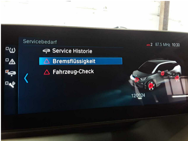
Damage #3: Braking system: Brake fluid - Due - Replace
