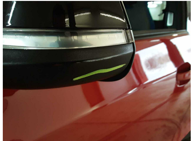
Damage #4: Wing mirror - right side: Cap - Scratched - Loss in value
