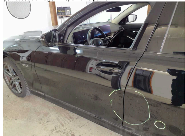
Damage #6: Door - front left side: Door - Dent / paintcoat damage - Repair and paint
