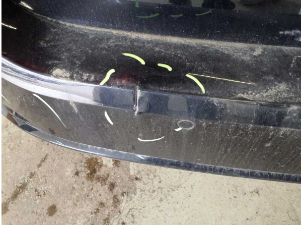
Damage #7: Rear bumper: Rear bumper - Dent / paintcoat dama... - Replace
