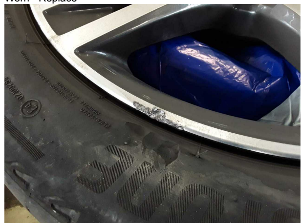
Damage #11: 2nd wheel set: 3 alloy rims - Scratched - Loss in value
