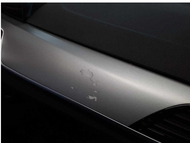
Damage #6: Interior: Interior (stark) - Soiled - Clean
