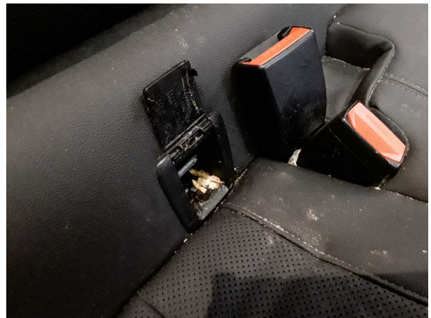
Damage #6: Interior: Interior (stark) - Soiled - Clean
