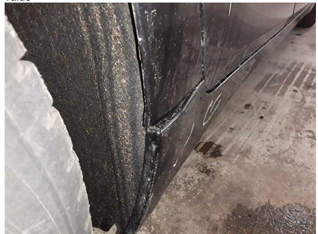
Damage #12: Sill - right side: Trim - Scratched - Replace
