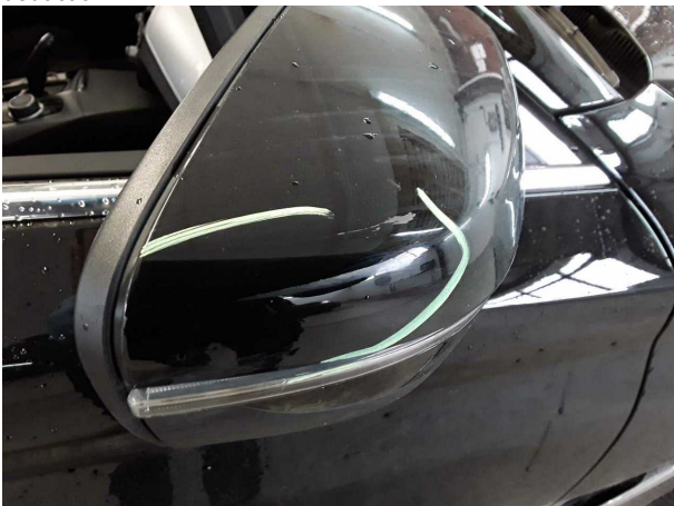
Damage #4: Wing mirror - right side: Cap - Scratched - Smart repair
