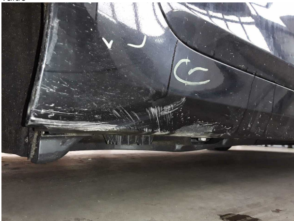
Damage #12: Sill - right side: Trim - Scratched - Replace
