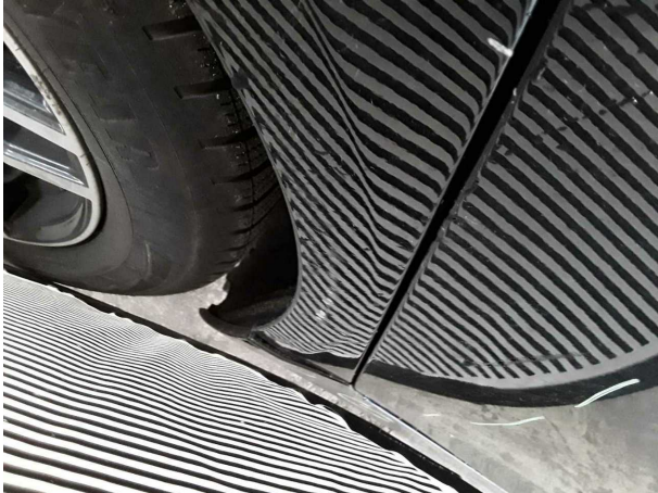
Damage #18: Side panel - rear right side: Side panel - Dent / paintcoat damage - Repair and paint
