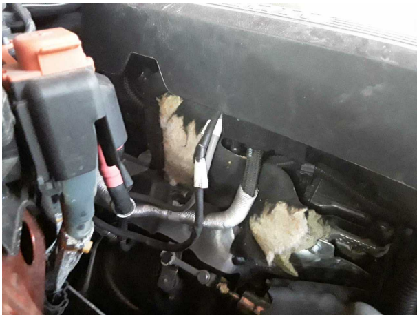
Damage #5: Engine: Engine cover - top / cover - Damage caused by marten / rodent - Replace
