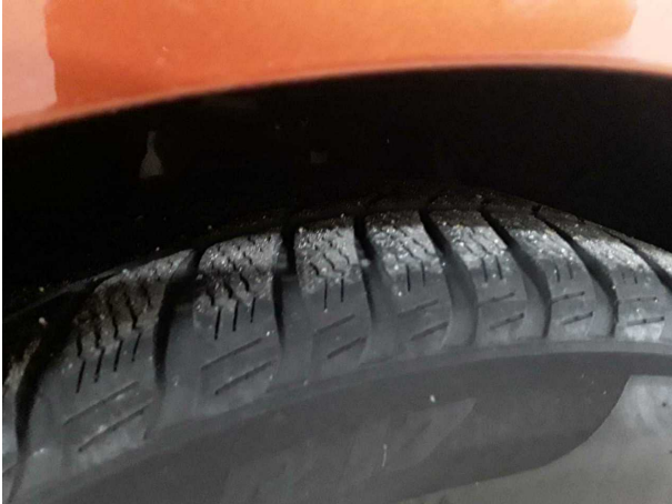
Damage #1: Wheel / tyres: Tyre - right - Worn - No deduction
