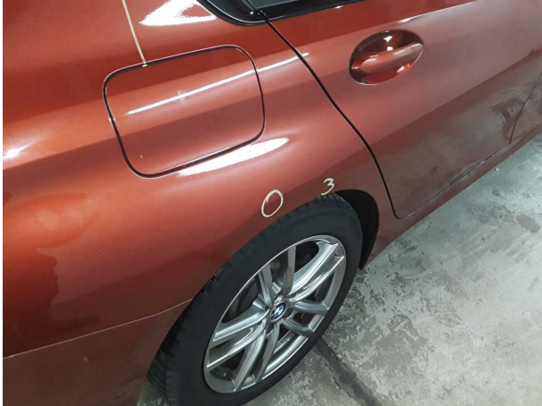
Damage #7: Side panel - rear right side: Side panel - Dent / paintcoat damage - Repair and paint
