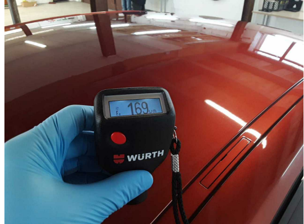
Repainting 1: Roof, Side panel - rear right side, Door - rear right side
