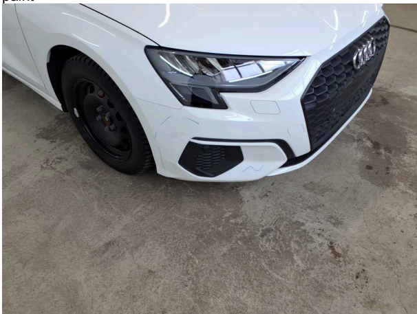
Damage #7: Front bumper: Front bumper - Scratched - Repair and paint
