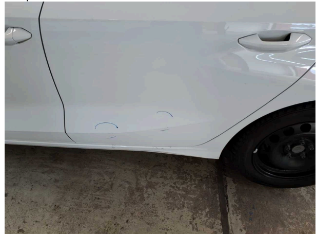
Damage #5: Door - rear left side: Door - Scratched - Repair a...
