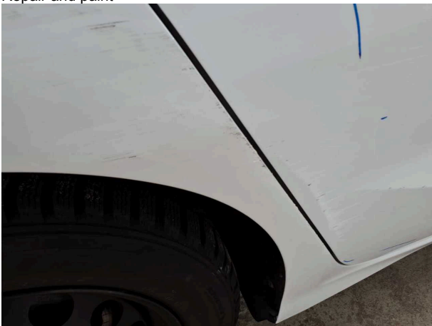
Damage #8: Side panel - rear right side: Side panel - Scratched - Repair and paint
