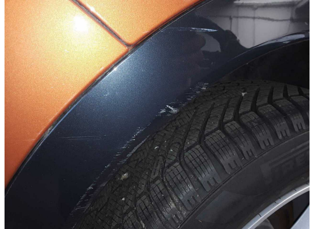
Damage #2: Side panel - rear right side: Wheel arch - Scratch(es) - Smart repair
