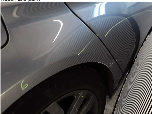
Damage #9: Side panel - rear right side: Side panel - Deformed - Repair and paint
