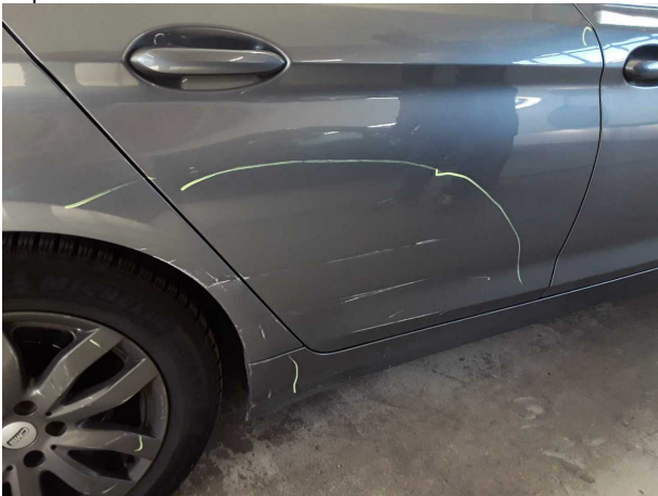
Damage #5: Sill - right side: Trim - Scratched - Repair and paint
