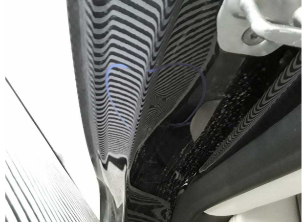
Damage #1: Side panel - rear right side: Sill - dent(s) - Smooth repair work
