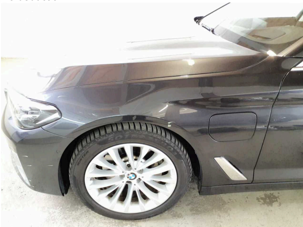
Damage #3: Mudguard - left side: Mudguard - left side - Scratch(es) - Cover / polish
