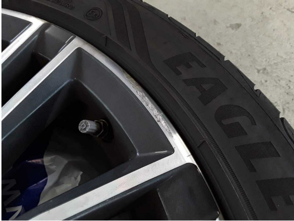
Damage #4: 2nd wheel set: 1 alloy rim - Scratched - Loss in value
