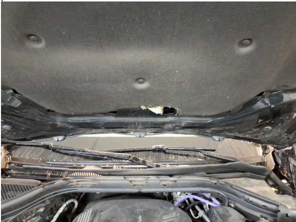
Damage #2: Bonnet: Insulation lining - Damage caused by marte... rodent - Replace
