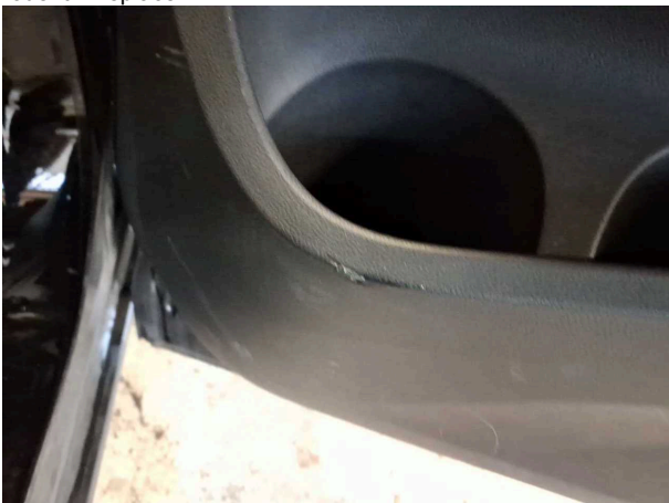
Damage #3: Trim / covers: Door trim - rear right side - Scratched - Loss in value
