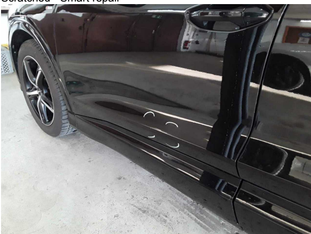
Damage #3: Door - front left side: Door - Scratched - Smart repair
