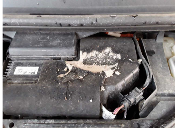
Damage #1: Engine: Engine cover - top / cover - Damage caused by marten / rodent - Replace
