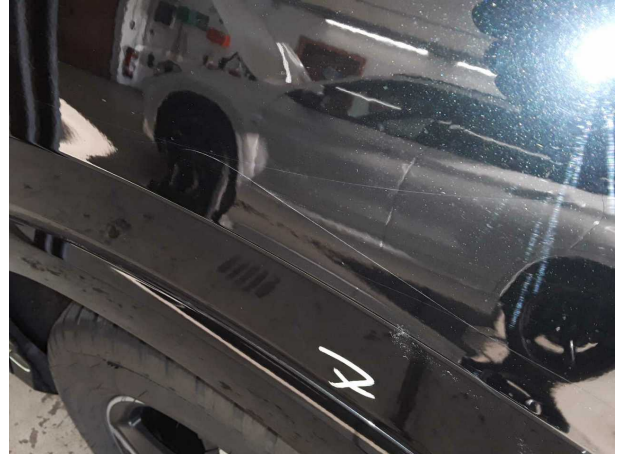
Damage #11: Side panel - rear left side: Side panel - Scratch... - Repair and paint
