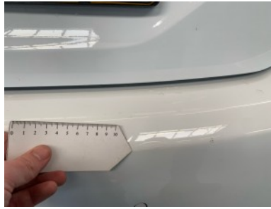
Rear bumper - Paint repair
