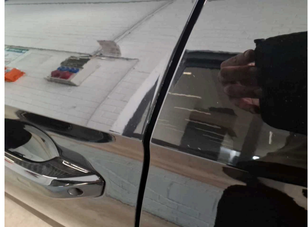
Damage #4: Door - front left side: Door edge - Scratched - Smart repair
