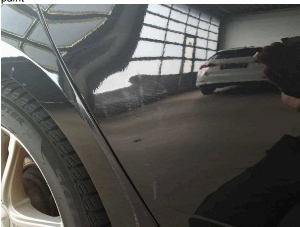
Damage #5: Door - rear right side: Door - Scratched - Repair and paint
