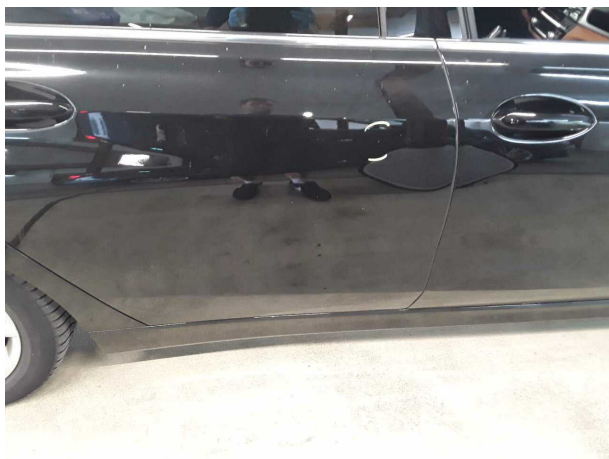
Damage #1: Door - rear right side: Door - Scratch(es) - Cover / polish
