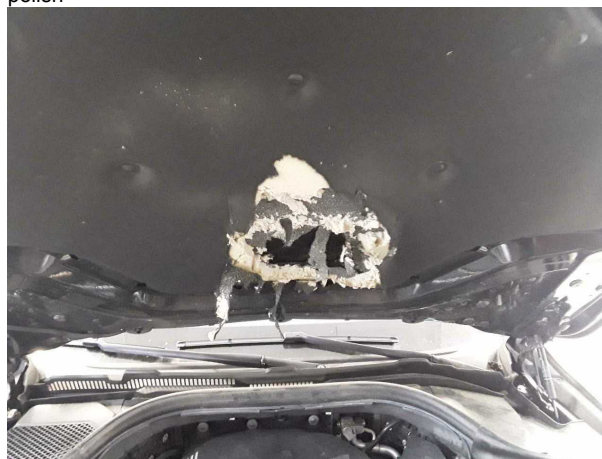
Damage #4: Bonnet: Insulation lining - Damage caused by marten / rodent - Replace
