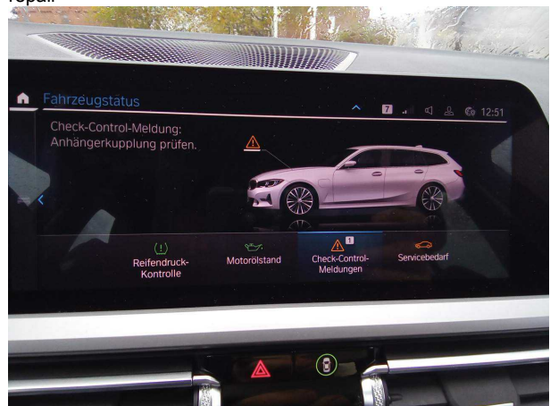
Damage #3: Instrument panel: Indicator light (AHK) - on - Diagnosed and repair if necessary
