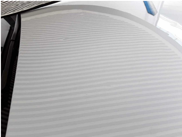
Damage #5: Bonnet: Bonnet (Hagelschaden ca. 50 Dellen) - dent(s) - Repair and paint
