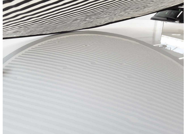
Damage #6: Roof: Roof (Hagelschaden, ca. 80 Dellen) - dent(...) - Repair and paint
