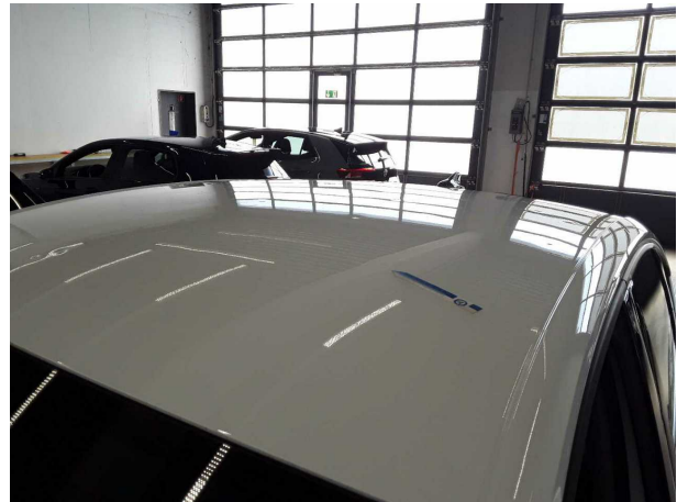
Damage #6: Roof: Roof (Hagelschaden, ca. 80 Dellen) - dent(s) - Repair and paint
