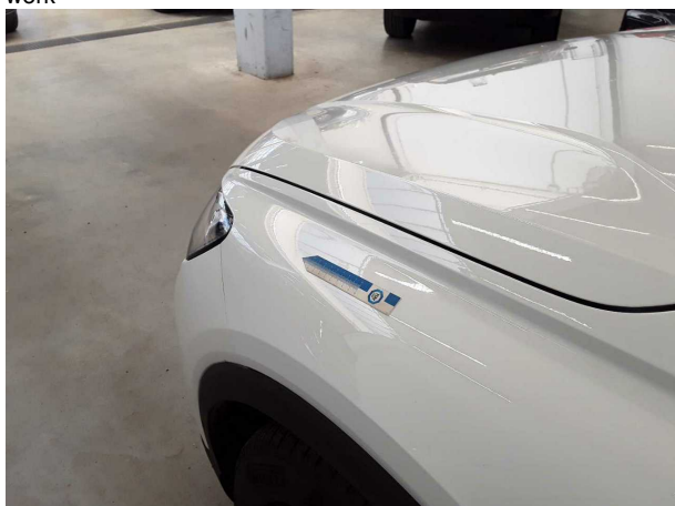
Damage #3: Mudguard - left side: Mudguard - left side - dent(s) - Smooth repair work
