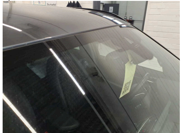
Damage #3: Vehicle glazing: Windscreen - Stone chips - Replace
