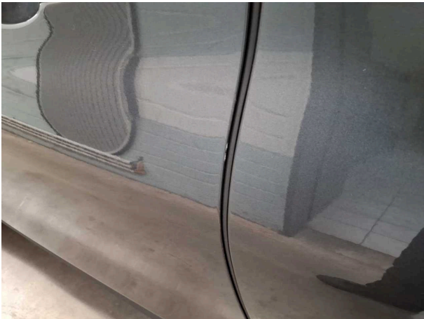
Damage #2: Door - front left side: Door edge - Scratched - Smart repair
