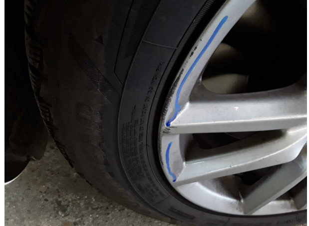
Damage #1: Wheel / tyres: Alloy rim - front left side - Scratched - Loss in value
