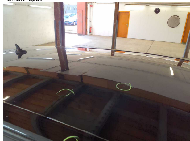
Damage #4: Roof: Roof - dent(s) - Smooth repair work
