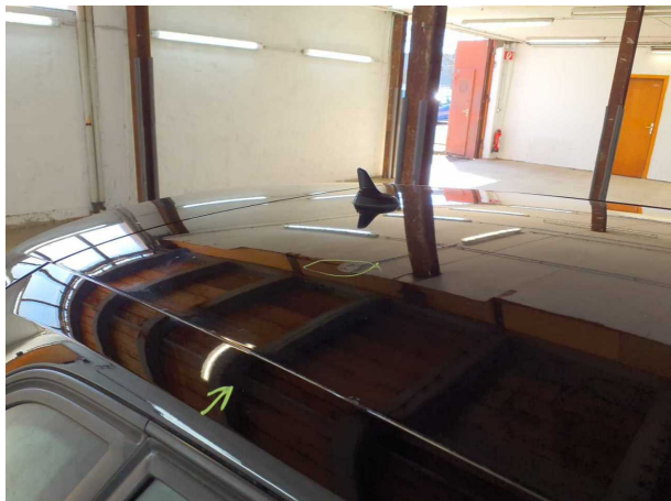
Damage #4: Roof: Roof - dent(s) - Smooth repair work
