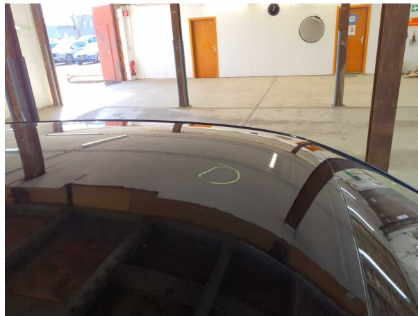
Damage #4: Roof: Roof - dent(s) - Smooth repair work
