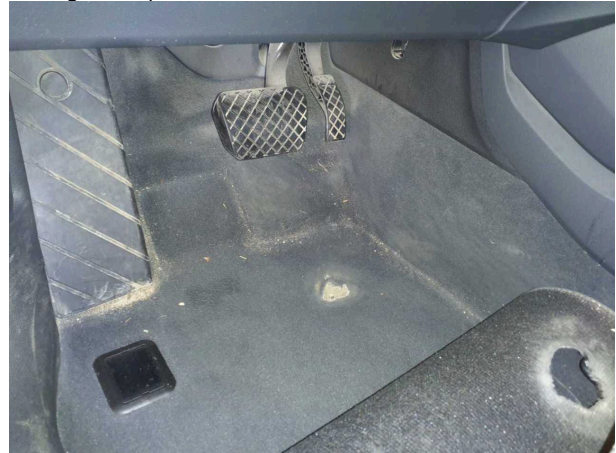
Damage #10: Trim / covers: Carpet - front left side - Damage... Replace
