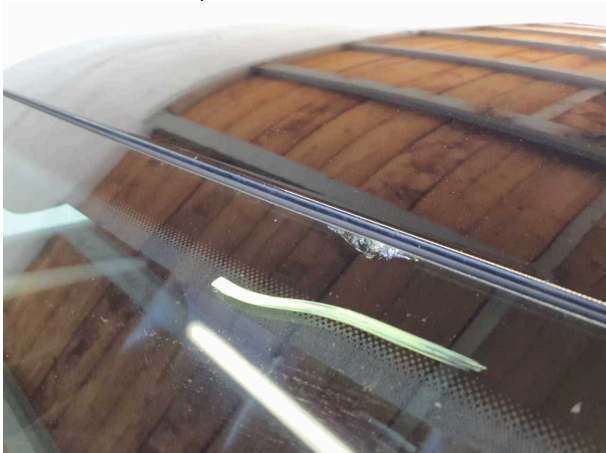
Damage #9: Vehicle glazing: Windscreen with rain sensor - Damaged - Replace
