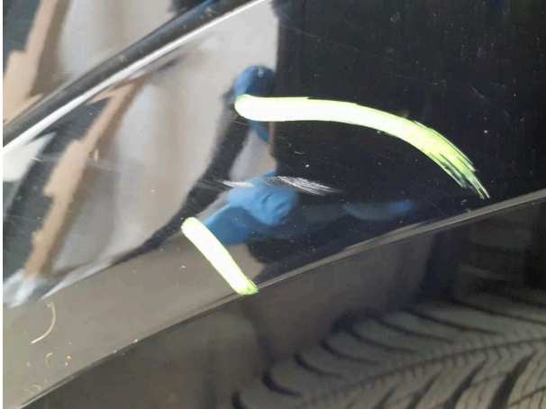
Damage #8: Side panel - rear right side: Wheel well extension - Scratched - Smart repair
