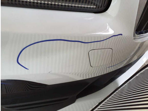
Damage #18: Front bumper: Front bumper - Deformed - Replace
