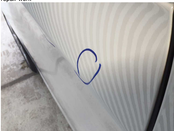
Damage #12: Door - rear right side: Door - Dent(s) - Smooth repair work
