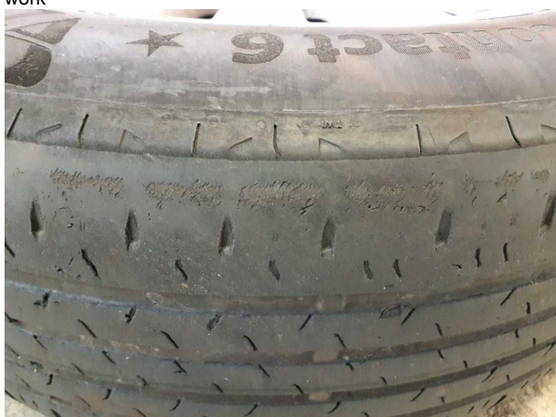
Damage #15: 2nd wheel set: 2 tyres (Vorne) - Worn - Replace
