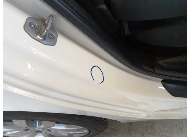
Damage #11: Side panel - rear right side: Sill - Dent(s) - Smooth repair work
