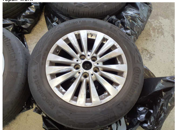
Damage #13: 2nd wheel set: 1 alloy rim - Scratched - Loss in value
