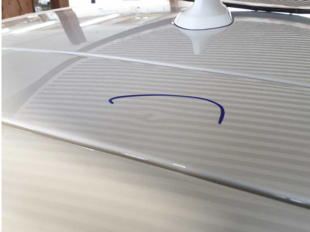
Damage #10: Boot lid / rear door: Boot lid - Dent(s) - Smooth repair work
