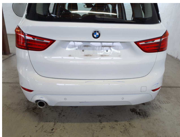
Damage #16: Rear bumper: Rear bumper - Scratched - Repair and paint
