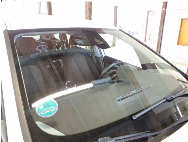
Damage #17: Vehicle glazing: Windscreen - Stone chips - Replace
