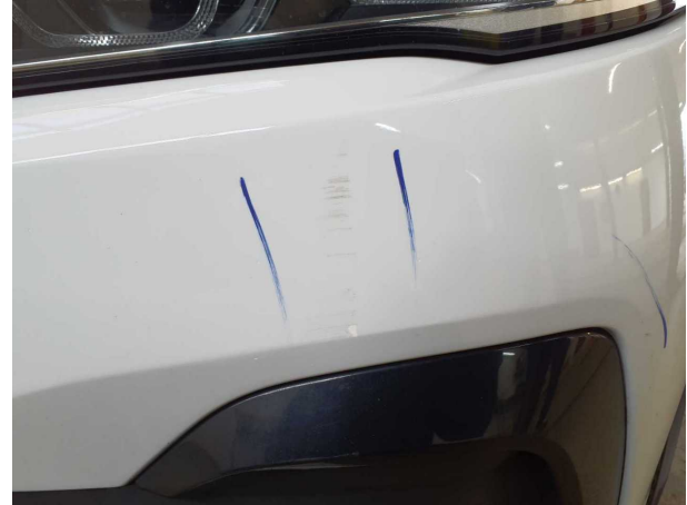
Damage #18: Front bumper: Front bumper - Deformed - Replace
