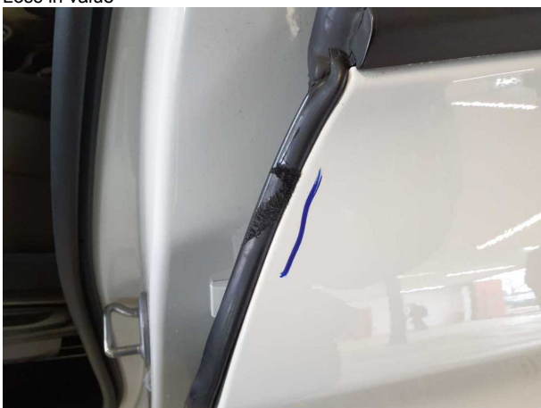
Damage #9: Door - rear left side: Door seal - Damaged - Replace
