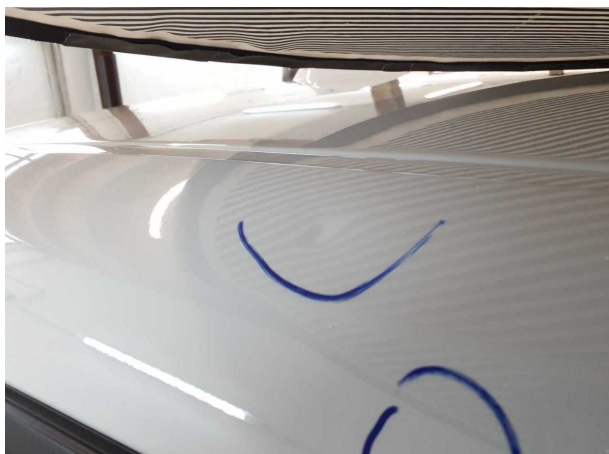
Damage #14: Roof: Roof rail - right side - Dent(s) - Smooth repair work
