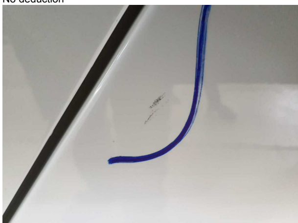
Damage #5: Side panel - rear left side: Side panel - Paint defect - Cover / polish
