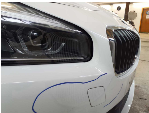
Damage #18: Front bumper: Front bumper - Deformed - Replace
