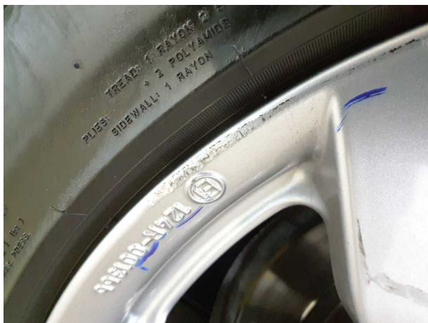
Damage #3: Wheel / tyres: Alloy rim - rear left side - Scratched - ... deduction
