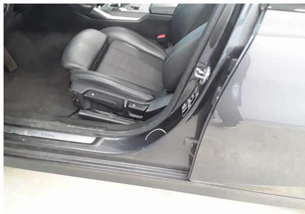
Damage #3: Sill - left side: Sill - Dent(s) - Smooth repair work
