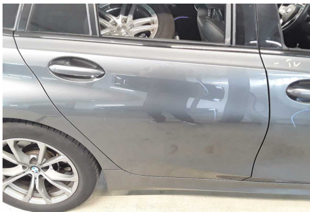
Damage #11: Door - rear right side: Door - Scratched - Repair and paint
