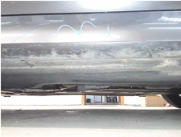
Damage #8: Sill - right side: Trim - Scratched - Smart repair
