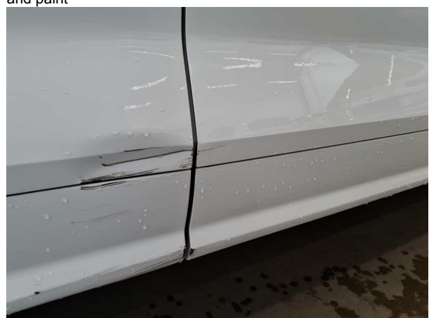
Damage #5: Door - front right side: Door - Scratched - Repair and paint
