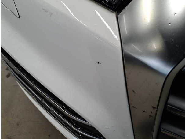
Damage #3: Front bumper: Front bumper - Scratched - Paint
