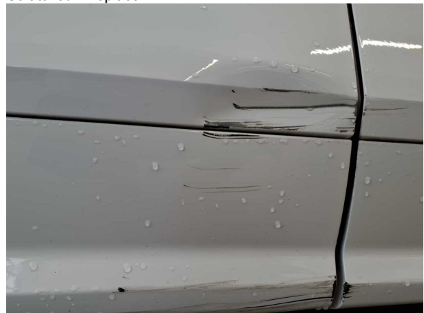
Damage #2: Door - rear right side: Brightware - lower - Scratched - Replace
