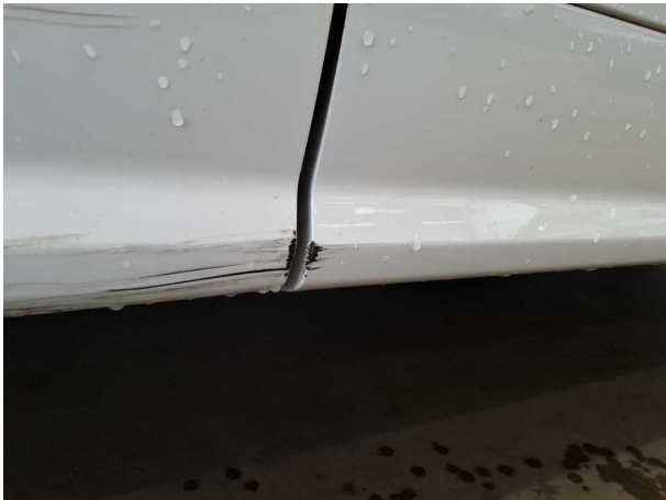
Damage #1: Door - front right side: Brightware - lower - Scratched - Replace
