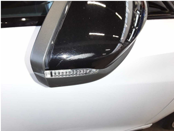
Damage #3: Wing mirror - right side: Mirror housing - Scratch(es) - Smart repair
