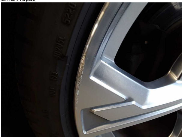
Damage #7: Wheel / tyres: Alloy rim - rear left side (Materialabtrag optisch zu hoch) - Scratched - Loss in value
