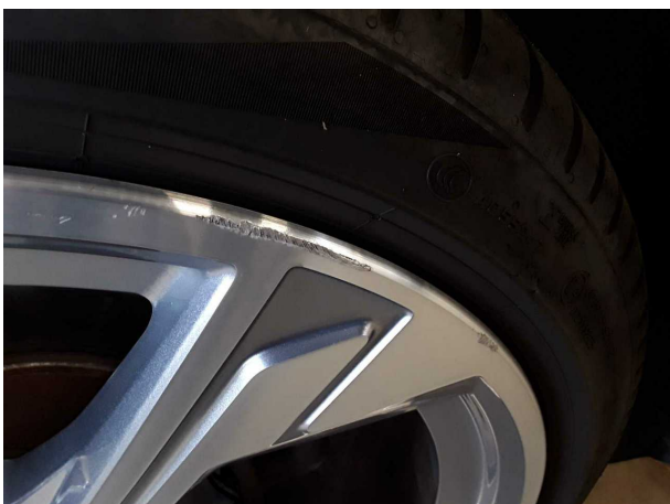
Damage #9: Wheel / tyres: Alloy rim - rear right side (Materialabtrag optisch gering) - Scratched - Loss in value
