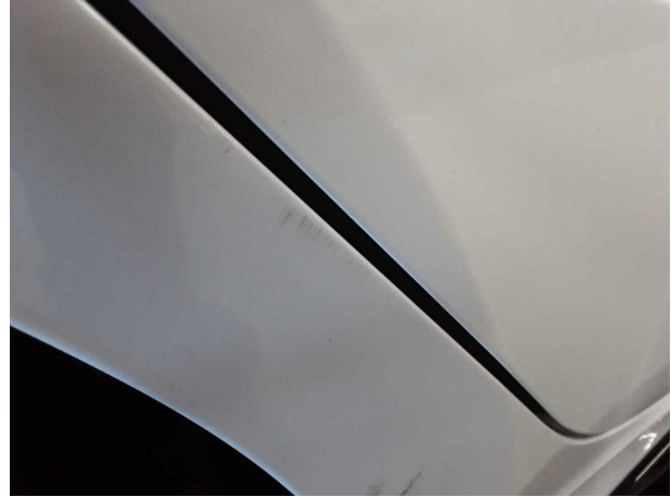
Damage #6: Side panel - rear right side: Wheel arch - Scratch(es) - Smart repair
