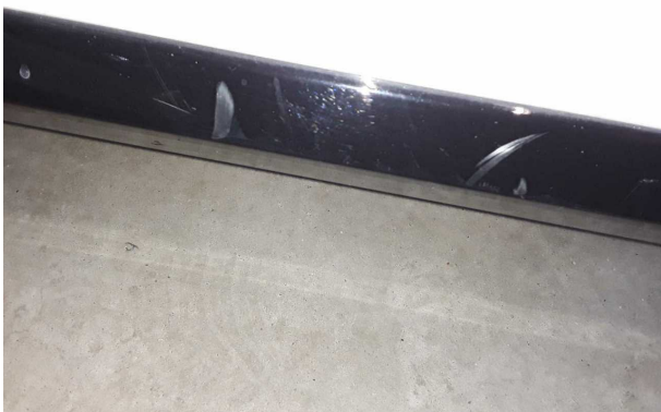
Damage #4: Sill - left side: Trim - Scratch(es) - Smart repair
