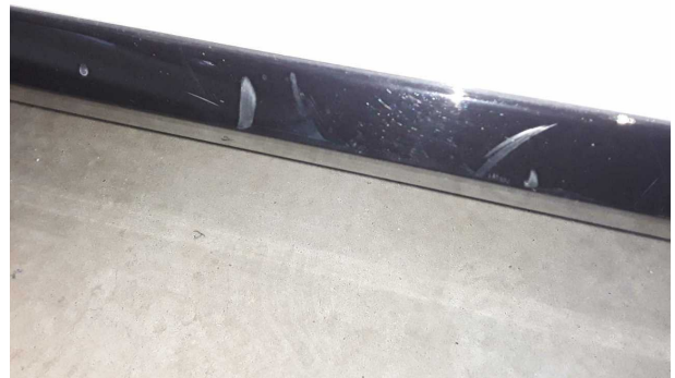
Damage #4: Sill - left side: Trim - Scratch(es) - Smart repair
