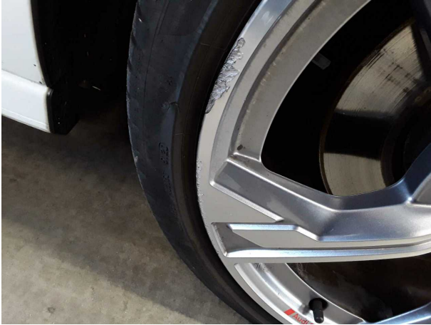
Damage #12: Wheel / tyres: Alloy rim - front right side (Materialabtrag optisch zu hoch) - Scratched - Replace
