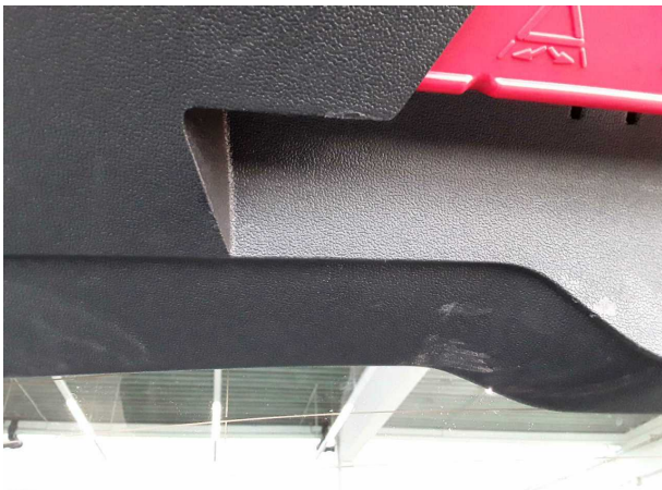
Damage #8: Trim / covers: Boot lining - Scratched - Loss in value
