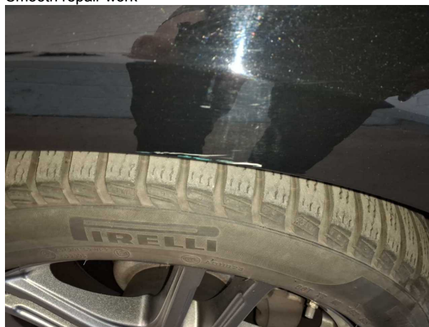
Damage #4: Mudguard - left side: Mudguard - left side - Scratched - Smart repair
