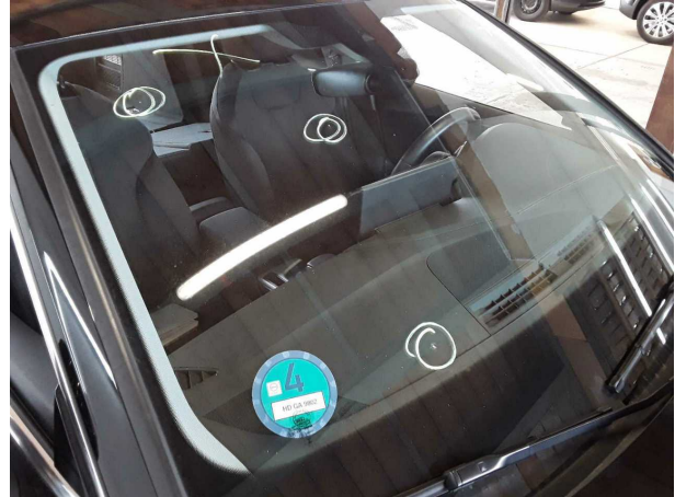
Damage #4: Vehicle glazing: Windscreen - Stone chips - Replace
