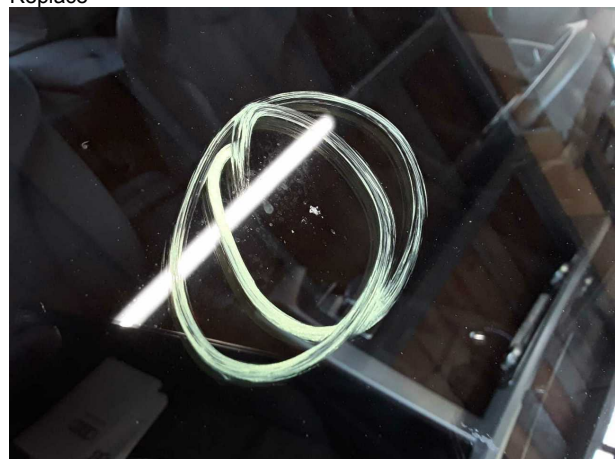
Damage #4: Vehicle glazing: Windscreen - Stone chips - Replace
