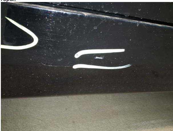
Damage #9: Sill - right side: Trim - Scratched - Repair and paint
