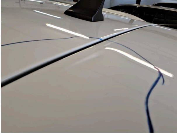
Damage #6: Boot lid / rear door: Rear spoiler - Dent / paintcoat damage - Replace
