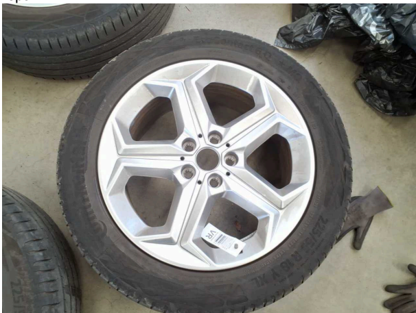
Damage #2: Wheel / tyres: Tyre - front left side - Broken / torn - Replace
