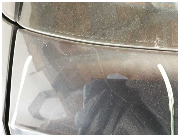
Damage #2: Boot lid / rear door: Boot lid - Scratch(es) - Cove... polish
