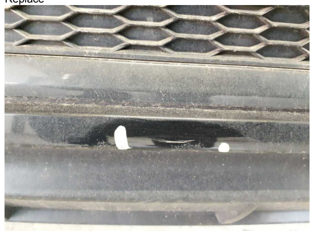
Damage #8: Rear bumper: Spoiler - Scratched - Replace
