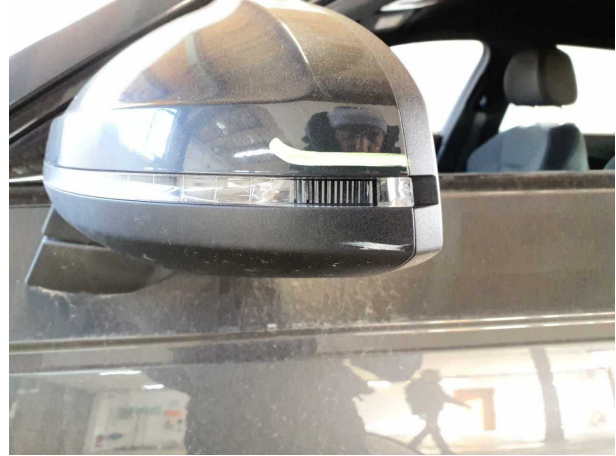
Damage #6: Wing mirror - left side: Mirror housing - Scratches... Loss in value
