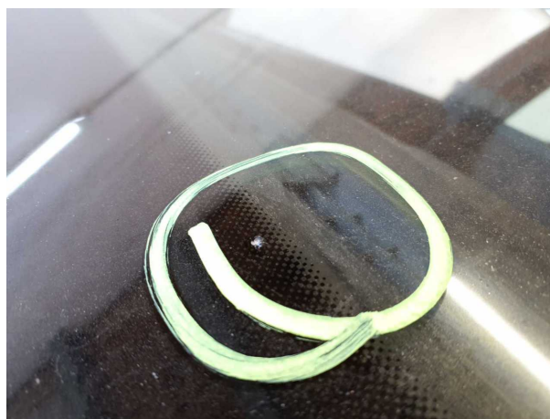
Damage #10: Vehicle glazing: Windscreen with rain sensor - Stone chips - Replace
