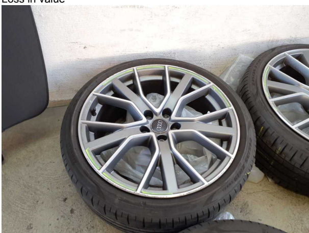
Damage #9: 2nd wheel set: Alloy rim set - complete - Scratched - Loss in value
