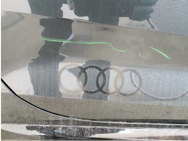
Damage #4: Door - rear right side: Door - Glued / labelled - De-glue / neutralise
