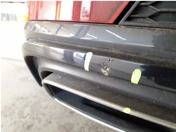
Damage #8: Rear bumper: Spoiler - Scratched - Replace
