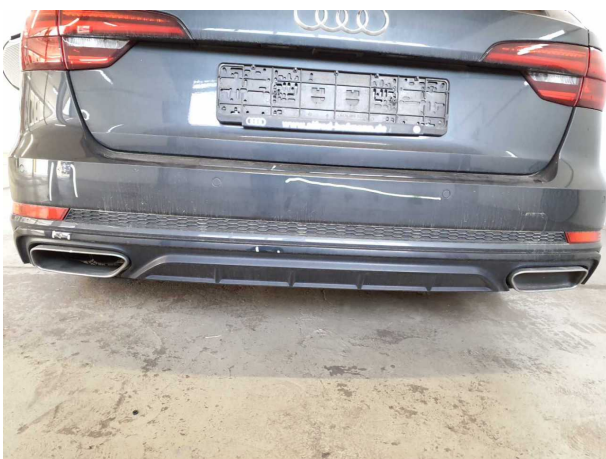
Damage #8: Rear bumper: Spoiler - Scratched - Replace
