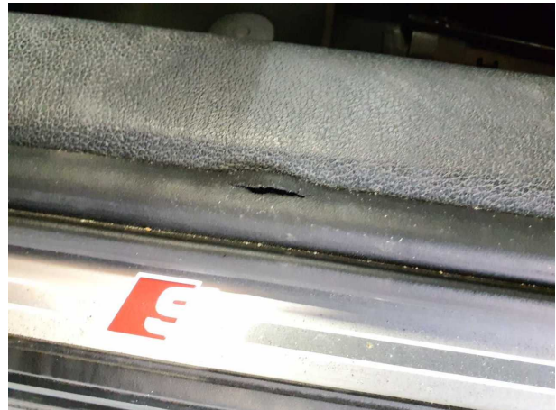
Damage #7: Body: Door seal - front left side - Damaged - Replace
