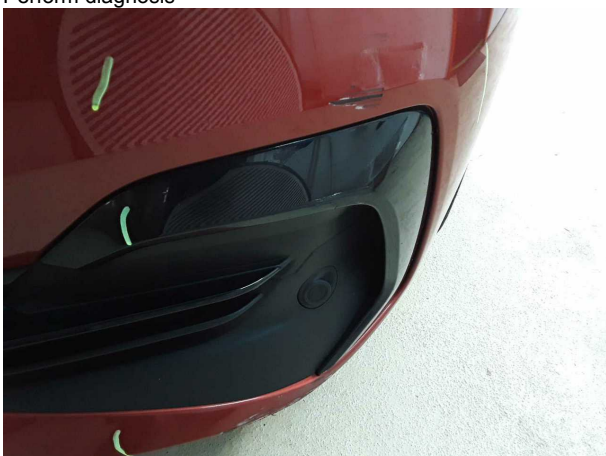
Damage #3: Front bumper: Spoiler - Scratched - Replace
