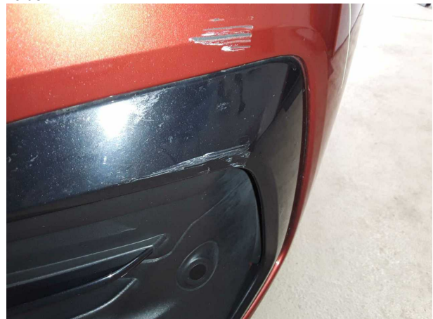
Damage #3: Front bumper: Spoiler - Scratched - Replace
