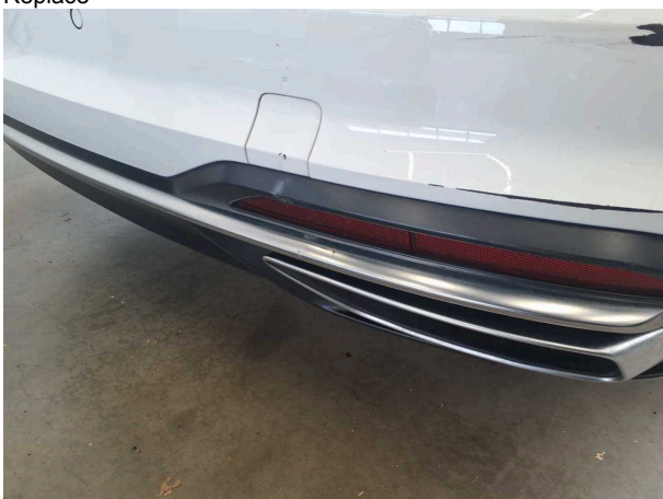
Damage #4: Rear bumper: Spoiler - Deformed - Replace
