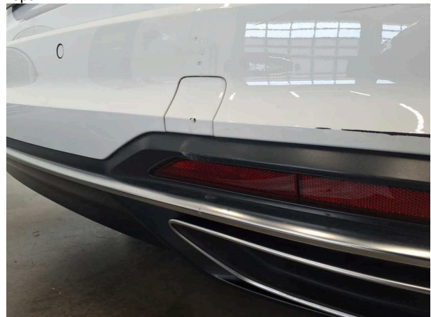
Damage #4: Rear bumper: Spoiler - Deformed - Replace
