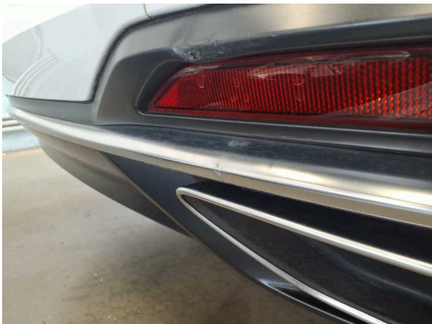
Damage #3: Rear bumper: Protection strip - centre - Scratched - Replace
