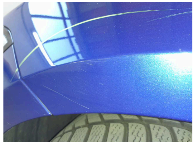
Damage #18: Mudguard - left side: Mudguard - left side - Scratched - Paint
