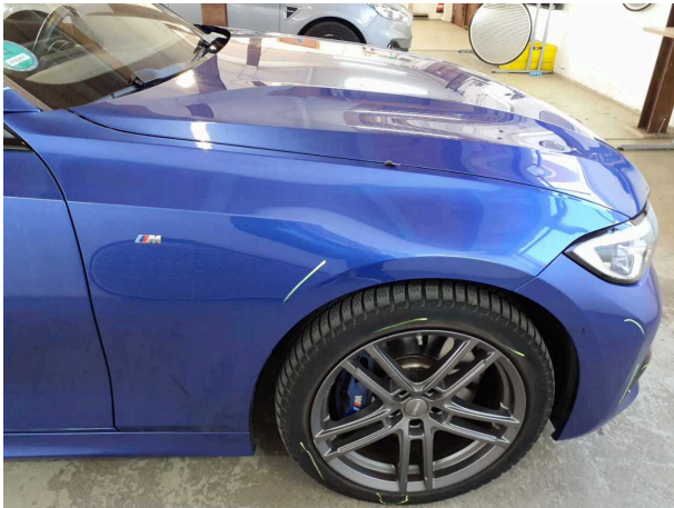
Damage #19: Mudguard - right side: Mudguard - right side - Scratch(es) - Paint
