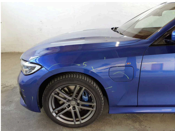
Damage #18: Mudguard - left side: Mudguard - left side - Scratch... - Paint
