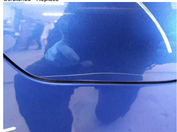
Damage #11: Fuel system: Tank cap - Scratched - Paint
