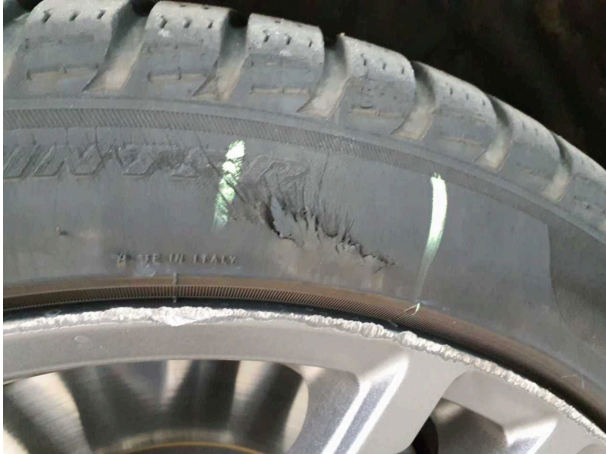
Damage #3: Wheel / tyres: Tyre - rear right side - Damaged - No deduction
