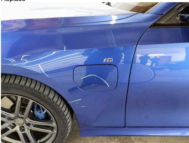
Damage #11: Fuel system: Tank cap - Scratched - Paint
