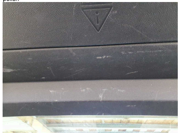
Damage #9: Trim / covers: Boot lid - interior trim - Scratched - Loss in value
