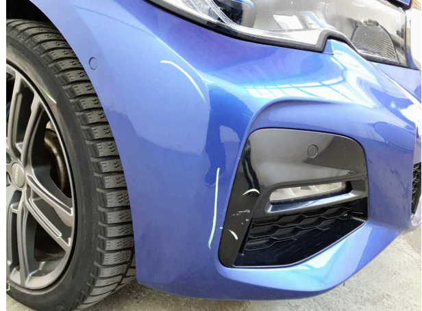
Damage #23: Front bumper: Front bumper - Scratched - Rep... and paint
