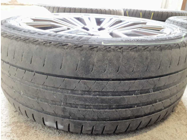
Damage #15: Front axle: Axles / undercarriage - Malposition - Set / adjust
