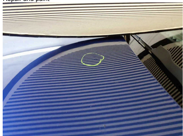
Damage #26: Bonnet: Bonnet - Dent / paintcoat damage - Repair and paint
