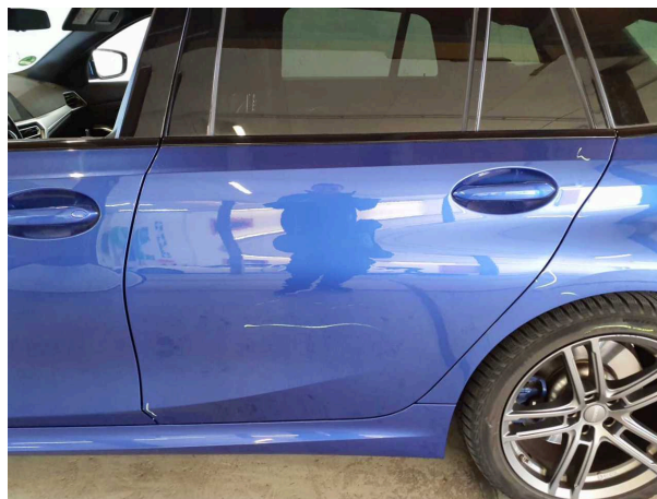
Damage #21: Door - rear left side: Door - Scratched - Paint
