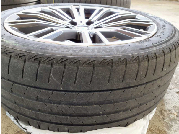
Damage #17: 2nd wheel set: 2 tyres - Worn - Replace
