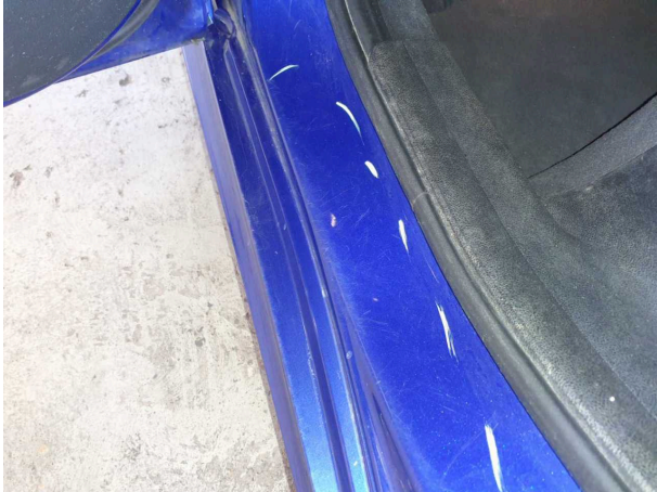
Damage #24: Side panel - rear left side: Side panel - Dent / paintcoat damage - Repair and paint
