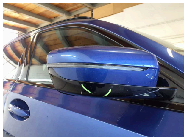
Damage #12: Wing mirror - right side: Mirror housing - Scratched - Smart repair
