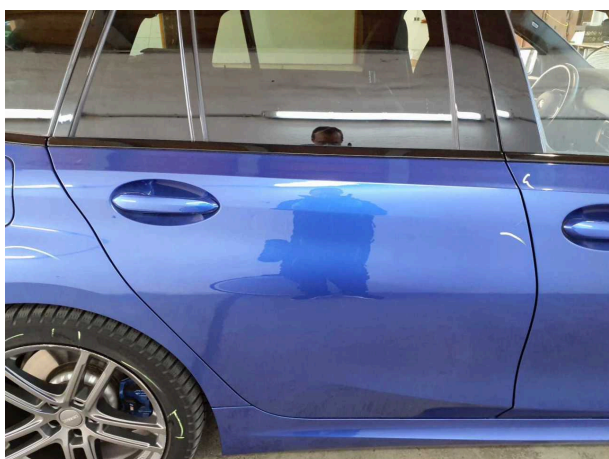
Damage #22: Door - rear right side: Door - Scratched - Paint
