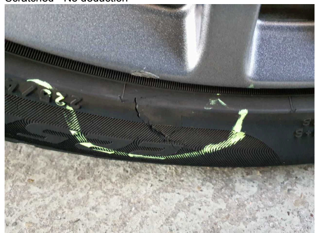
Damage #5: Wheel / tyres: Tyre - front right side - Damaged - No deduction
