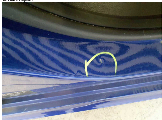
Damage #14: Sill - right side: Sill - Dent / paintcoat damage - Smart repair
