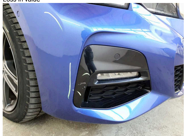
Damage #10: Front bumper: Cover bumper - front (Vr) - Scratched - Replace
