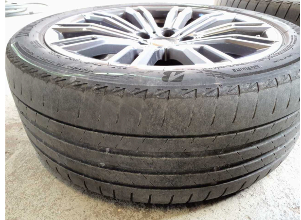
Damage #17: 2nd wheel set: 2 tyres - Worn - Replace
